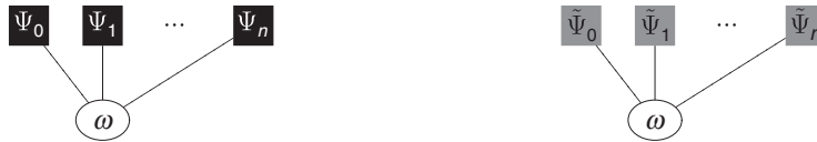
Expectation Propagation. Figure 1. (left-hand side) A so-called factor graph corresponding to the i.i.d. assumption in Bayesian machine learning. Each box corresponds to a factor or term. A circle corresponds to a variable. Factors are connected to the variables that they contain. \Psi_0 corresponds to the prior, \Psi_1 \dots \Psi_n are the likelihood terms for the n data points. (right-hand side) Factor graph of the approximating distribution. The original terms have been replaced by term approximations
