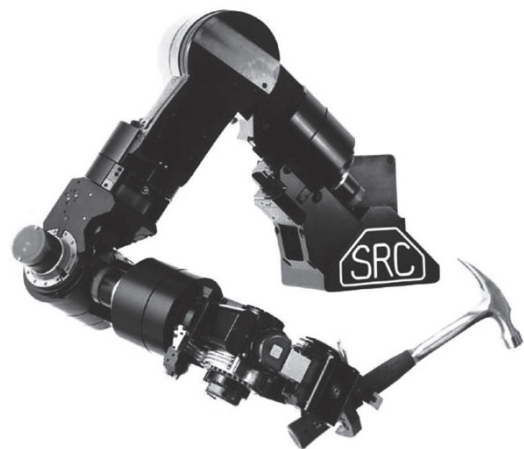
b Seven Degree-of-Freedom Sarcos Robot Arm
