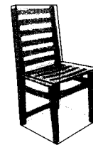
Figure 12.8. A chair can be modeled using a pair of interconnected box shapes.
