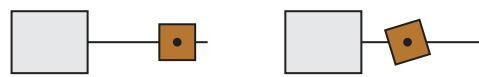
Figure 13.17 Groove joint: Object B moves and rotates along a groove on object A
