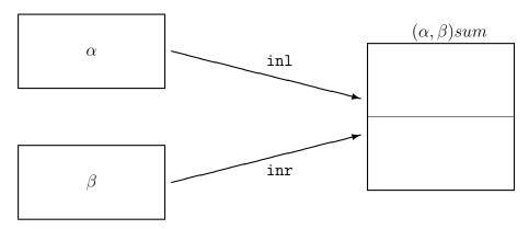
This is similar to a union in C, but in ML the copies of the component types are kept apart and one always knows which of these an element of the union belongs to. By contrast, in C the component types are overlapped, and the programmer is responsible for this book-keeping.
