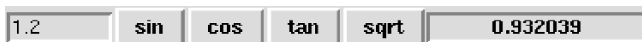
Fig. 6.10. GUI to be developed in Exercise 6.1. The GUI consists of an entry field, four buttons, and a label (with sunken relief).
