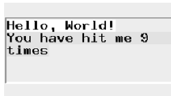
Fig. 11.5. Example on binding mouse events to modifications of a text in a text widget.
