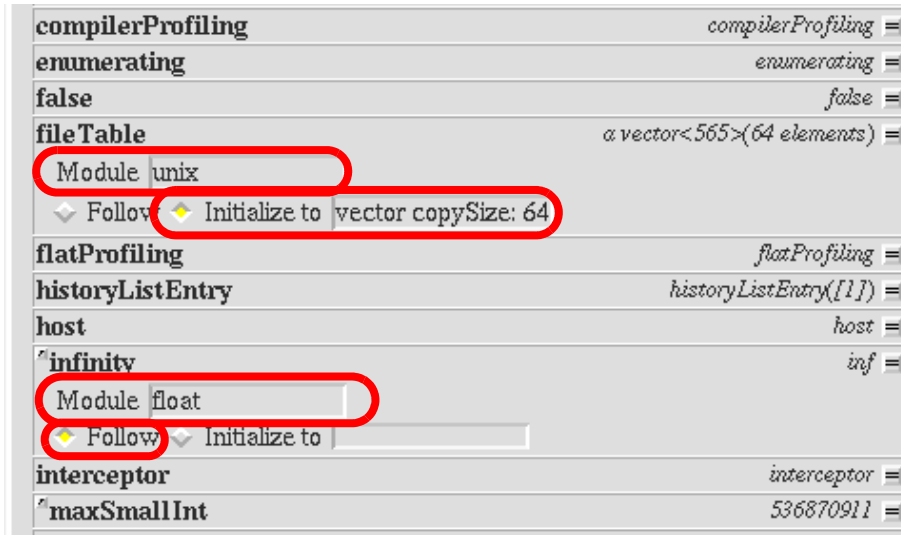
Figure 24. Annotations for transporting slots. The ovoid outlines have been added to show the module and initialization information for two slots (named fileTable and infinity ) in a Self object.
