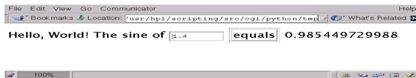
Fig. 7.3. An improved Web interface to our Scientific Hello World program ( hw2.py.cgi script).
