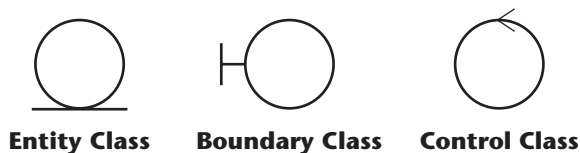
Figure 11.1 UML stereotypes (extensions of UML) for representing an entity class, a boundary class, and a control class.
