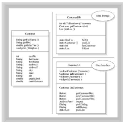
Figure 7.9 Partitioning the Customer class
