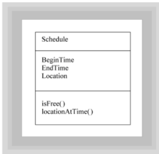
Figure 6.18 Class diagram of the Schedule class
