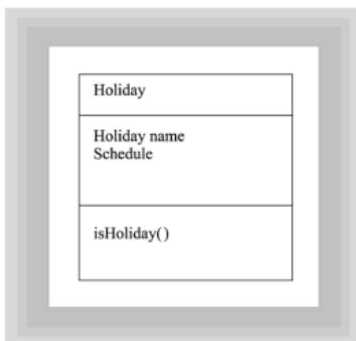
Figure 6.17 Class diagram of the Holiday class
