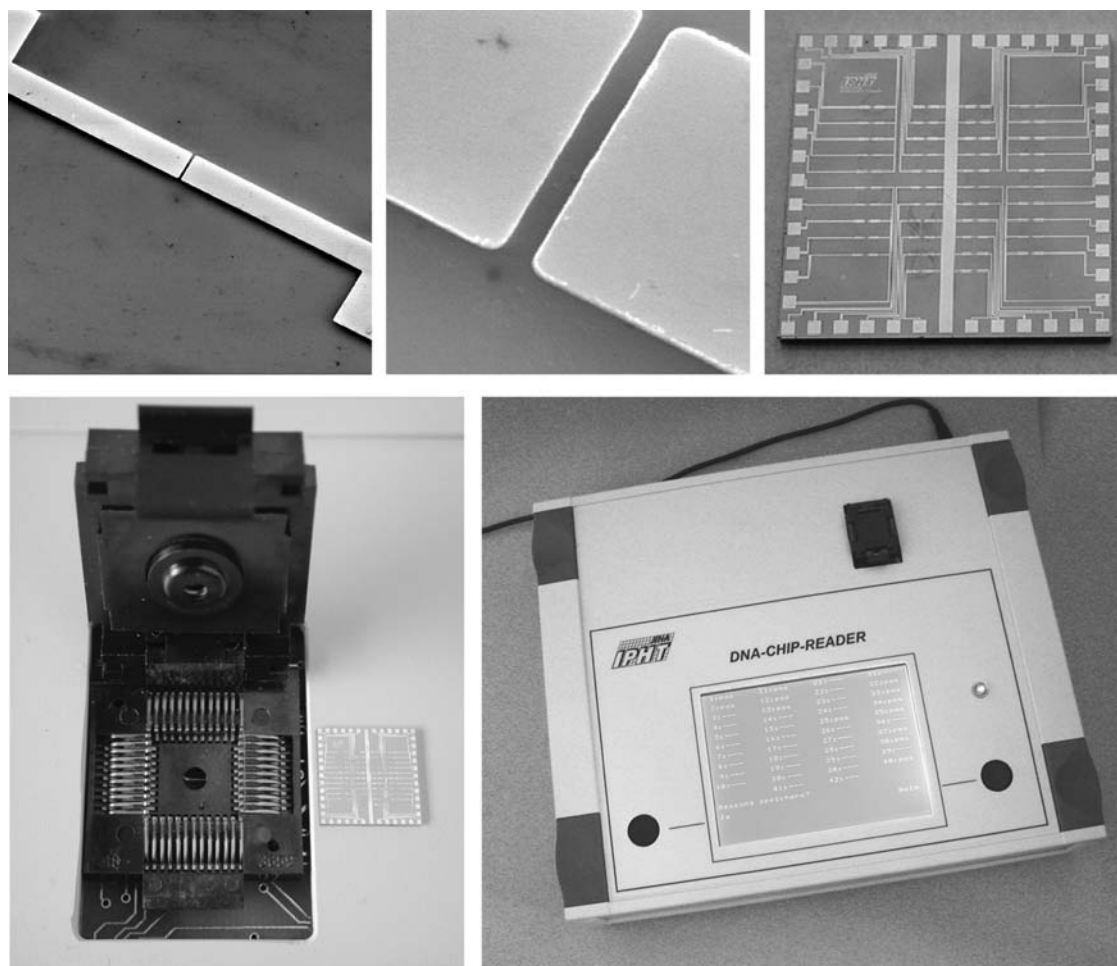
Fig. 6 System for electrical readout of DNA hybridization. [18] Top row: An array of micrometer-sized gaps (left, center) of microstructured gold electrodes for DNA detection (cf. Fig. 5C) is arranged on a half-inch chip (right). Bottom row: A chip holder (left) is part of the reader (right) that contains measurement electronics controlled by an embedded PC. © 2003 American Institute of Physics.
