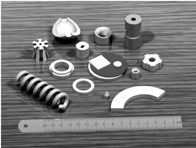
Fig. 10 Ceramic articles synthesized by ultrasonic pressing of nanopowders. Source: From Ref. [19] .
