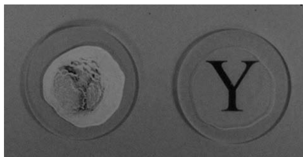
Fig. 5 Thin films prepared from hydrosols of Aldrich zeolite Y (left) and nanocrystalline zeolite Y (right).
