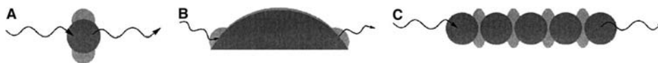
Fig. 1 Incident light on nanostructured metal surfaces can result in localized (standing) plasmon resonances (A), propagation of surface plasmon waves (B), or a combination of the two (C). Excitation of conduction electrons produces local electromagnetic fields (pink) near the metal surfaces.
