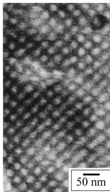
Fig. 10 Transmission electron micrograph of a strongly segregated E/SEB diblock copolymer that exhibits confined crystallization . The spherical melt microdomains are exactly preserved on crystallization despite the presence of a rubbery matrix. Source: From Ref. [37] , © 2000 American Physical Society.
