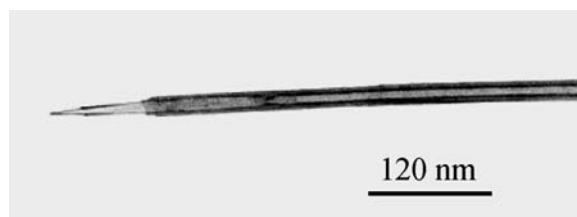
Fig. 10 The tip-shape termination of the WS 2 nanotube associated with the change of the chirality.
