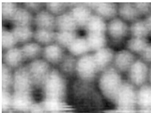
Fig. 1 Atomic resolution image ( 4 \times 2.5 nm) of the force gradient across a Si(111)-(7 \times 7) surface. Round “bumps” correspond to single atoms. Measured with a subresonance AFM at an ultrasmall lever amplitude of 0.25 Å. Feedback was maintained via the tunneling current.
