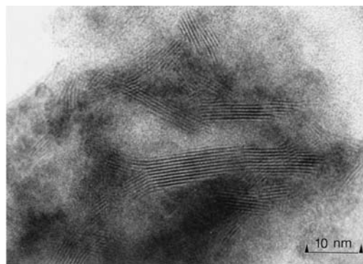
Fig. 17 SnS_2 filaments, synthesized at 200°C. The lattice fringes distance is 0.56 nm, corresponding to the \{0002\} planes. The filaments have a length of around 30 nm and a width of 3–4 nm. Source: From Ref. [43] .
