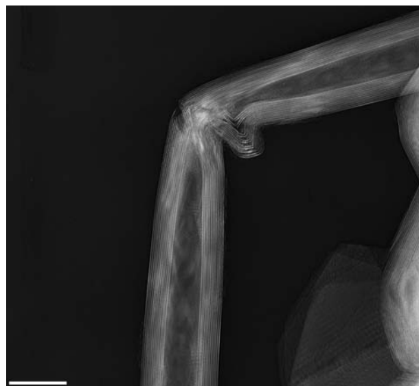
Fig. 4 TEM image of a naturally buckled nanotube. This image demonstrates clearly that the cross-section of the nanotube is not constant (bar 20 nm). Source: Adapted from Ref. [25] .
