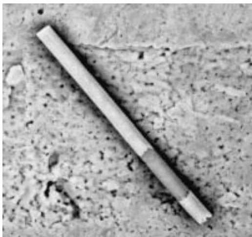
Fig. 2 Field emission SEM image of a AuAuAgAu nanowire, acquired with backscattered electron detection. The Ag segment appears darker as compared to the Au.
