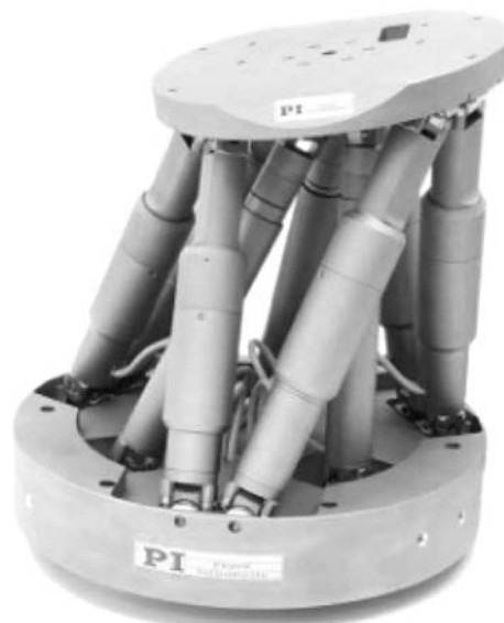
Fig. 2 Nanometer scale Stewart platform manipulator (left picture—©K.E. Drexler, Institute of Molecular Manufacturing— http://www.imm.org ) and macroscopic commercial counterpart (right picture—by Physik Instrumente GmbH). Both designs trade off controllability (highly coupled designs that limit speed), dexterity (useful in obstacle avoidance), and reachable workspace for higher payload.
