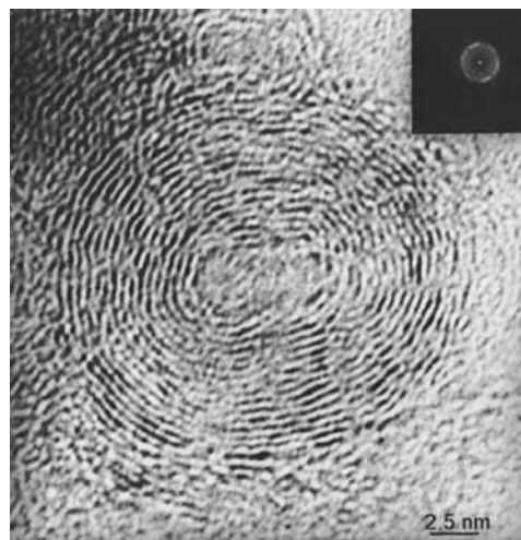
Fig. 3 High-resolution transmission electron microscopy image of MoS 2 Onion-like structure. Fourier transform of the structure is shown in the inset. Source: From Ref. [11] .
