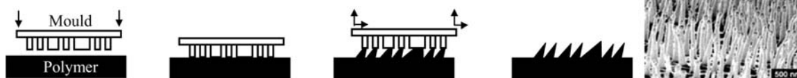
Fig. 8 Fabrication of structured surfaces by fiber drawing method. The SEM picture shows an example of obtained PMMA fibrillar surface. Source: Reprinted with permission from Ref. [34] .
