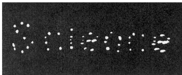
Fig. 9 The word “science” formed using STM nanolithography. Source: From Ref. [59] . © (1995) American Chemical Society.
