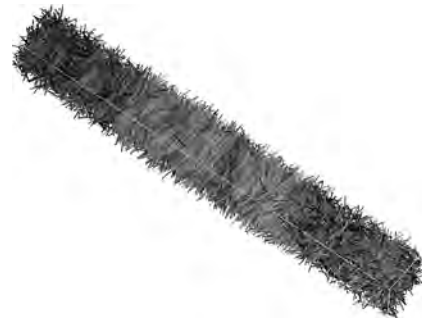
Figure 22. The image shows a snapshot from a Monte Carlo simulation of long, thin molecules in an elongated periodic box. The molecules are color-coded by orientation. The system shows two phases at equilibrium: a nematic liquid crystal (in the center) and an isotropic liquid (on either side) separated by planar interfaces. These simulations allowed the first determination of the surface tension of the equilibrium nematic–isotropic interface and confirmed that the molecules in the nematic phase are preferentially aligned in the plane of the surface. Subsequent simulations, using the molecular dynamics method, investigated capillary-wave fluctuations of this interface as a function of cross-sectional area.
