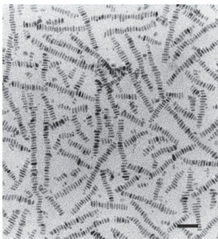
Figure 33. TEM image showing ordered chains of prismatic \text{BaSO}_4 nanoparticles prepared in AOT microemulsions at [\text{Ba}^{2+}]:[\text{SO}_4^{2-}] molar ratio = 1 and w = 10 . Scale bar = 50 nm. Reprinted with permission from [25], M. Li et al., Nature 402, 393 (1999). © 1999, Macmillan Magazines Ltd.
