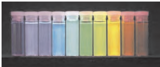
Figure 1. Ten different emission colors of different size ZnS-coated CdSe nanoparticles excited with a near-UV lamp. From left to right (blue to red), the emission maxima are 443, 473, 481, 500, 518, 543, 565, 587, 610, and 655 nm, respectively. Reprinted with permission from [1], M. Y. Han et al., Nature Biotechnol. 19, 631 (2001). © 2001, Macmillan Magazines Ltd.
