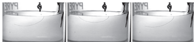
Figure 7. Electromechanical actuation of a HiPCO SWNT spun fiber in an electrolyte solution (NaCl 1 M) when an alternative voltage of 1 V is applied at a frequency of 1 Hz. It exhibits a periodic motion as shown in the pictures.
