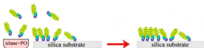
Figure 2. Schematic showing the method of preparing molecular gradient by vapor deposition of organosilanes onto hydrophilic substrates.
