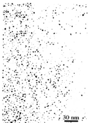
Figure 3. TEM image of a stable PVP-protected Pt nanocluster with a high Pt/PVP ratio (monomeric unit of PVP/Pt mole ratio: 0.35) prepared by dissolving a precipitate of “unprotected” Pt nanoclusters. The average diameter of the Pt nanoparticles is 1.5 nm. Reprinted with permission from [88], Y. Wang et al., Chem. Mater. 12, 1622 (2000). © 2000, American Chemical Society.
