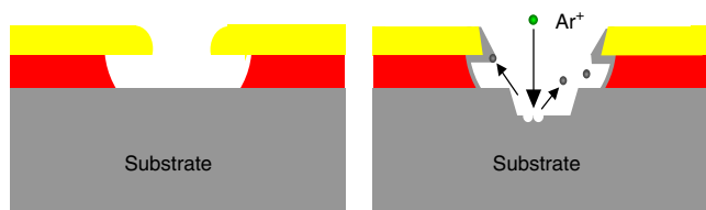
Figure 89. Resputtering of material in physical plasma etching.
