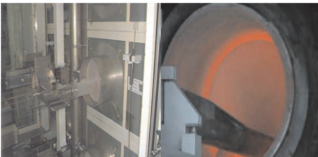
Figure 61. Thermal oxidation furnace.
