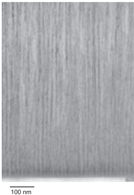
Figure 34. Cross-sectional SEM image of a Ni-nanowire array, which was electrochemically deposited and embedded into nanopores of alumina membranes. We prepared arrays with three different mean pore diameters of about 30, 55, and 96 and with the same pore length of 2 \mu\text{m} for this work. This nanowire at least has the following three advantages. high purity, good surface morphology, and no surface oxidation. The first advantage arises from the electrochemical deposition and leads to reduction of scattering probabilities by impurities and defects. The second and third advantages arise from embedding the nanowires into the nanopores with good morphology of the inner walls and lead to reduction of probabilities of surface-spin scattering due to bad morphology and surface oxidation. Spin-flip scattering and spin fluctuation caused by such parasitic factors (i.e., impurities, defects, and poor surface morphology) lead to drastic reduction of phase coherence in ferromagnetic nanowires in an essential way. Hence, our special wire structure is relevant to realize coexistence of mesoscopic phase coherence and ferromagnetism. Magnetic field was applied along with the wire axis in all the measurements in this work.
