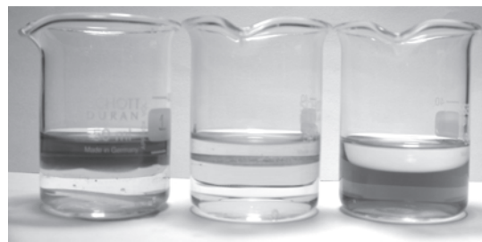
Figure 1. Nanocrystalline film of Au formed at the toluene-water interface (middle). Gold is introduced as a toluene solution of \text{Au}(\text{PPh}_3)\text{Cl} while partially hydrolyzed THPC (tetrakis(hydroxymethyl)phosphonium chloride) in water acts as a reducing agent. The film is obtained when the two layers are allowed to stand for several hours. When dodecanethiol is added to the toluene layer, the film breaks up forming an organosol (left) while mercaptoundecanoic acid added to water produces a hydrosol (right).
