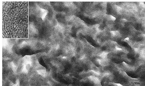
Figure 4. Representative TEM micrograph of PODS-Pd including Pd nanoparticles derived from \text{Na}_2\text{PdCl}_4 and embedded within the siloxy bilayers of the PODS lamellar nanostructure. The 3\times enlargement more clearly displays the nanoparticles within their host medium. Reprinted with permission from [38], L. M. Bronstein et al., Langmuir 16, 8221 (2000). © 2000, American Chemical Society.
