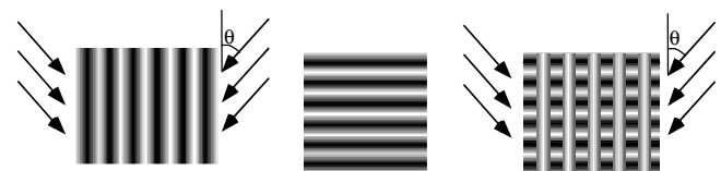
Figure 23. Left: first exposure of the substrate with the photolacquer layer. Middle: rotation of the substrate 90^\circ . Right: second exposure of the substrate.
