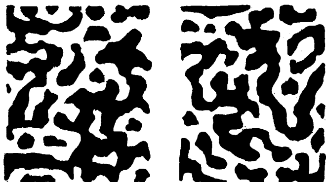
Figure 1. Model of porous structure for porous glass.
