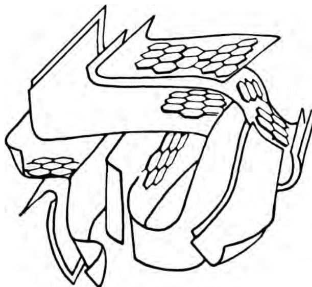
Figure 16. A conceptual model of porous carbon. This is a three-dimensional representation of Figure 1a. Reprinted with permission from [46], R. C. Bansal et al., in Active Carbon , Chapter 3. Dekker, New York, 1998. © 1988, Dekker.
