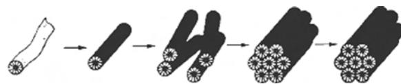
Figure 3. Self-assembly of silicate-encapsulated micelle rods into hexagonal mesophase. Reprinted with permission from [4], J. Y. Ying et al., Angew. Chem. Int. Ed. Engl. 38, 56 (1999). © 1999, Wiley.
