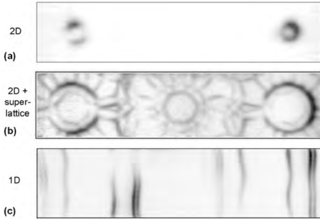
Figure 29. Fermi surfaces of two- and one-dimensional surface states on silicon, obtained by angle-resolved photoemission with energy and angle multidetection. The x- and y-axes are the \mathbf{k} -vector components parallel to the surface, with \mathbf{k} = 0 at the center. A truly one-dimensional Fermi surface would consist of vertical lines since the energy does not depend on the wave vector perpendicular to the chains (vertical). (a) Si(111) \sqrt{3} \times \sqrt{3} -Ag (see Fig. 28) with a few percent excess Ag forming small electron pockets. (b) Si(111) \sqrt{21} \times \sqrt{21} -(Ag+Au) with a superlattice of Au atoms on top of the \sqrt{3} \times \sqrt{3} -Ag lattice forming large Fermi circles. The \sqrt{21} \times \sqrt{21} superlattice causes faint replicas of the Fermi circles. (c) Si(553)-Au, a nearly one-dimensional structure containing a single Au chain per unit cell. Adapted with permission from [339], J. N. Crain et al., Phys. Rev. B 66, 205302 (2002) (a), (b); and from [362], J. N. Crain et al., Phys. Rev. Lett. 90, 176805 (2003) (c). © 2002 and 2003, American Physical Society.
