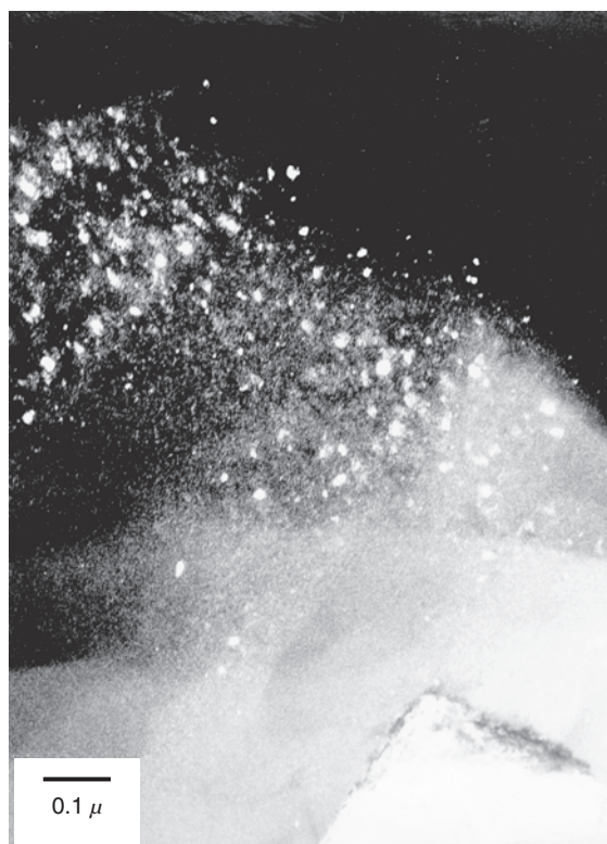
Figure 5. TEM micrograph (dark-field) of spherical Si nanocrystals in porous Si. Reprinted with permission from [61], A. Nakajima et al., Appl. Phys. Lett. 62, 2631 (1993). © 1993, American Institute of Physics.
