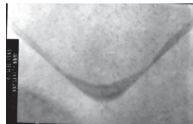
Figure 5. TEM image of the cross section of an \text{In}_{0.2}\text{Ga}_{0.8}\text{As}/\text{Al}_{0.5}\text{Ga}_{0.5}\text{As} QWR.
