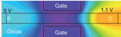
Figure 1.15 Electrostatic potential in a double-gate transistor with 30-nm gate length and 10-nm Si thickness; V_g = 0 \text{ V} ; V_d = 1.1 \text{ V} ; midgap gate material.
