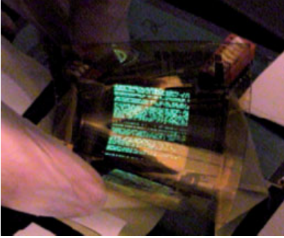
Figure 6.25 A flexible 48 \times 48 pixel active-matrix organic light-emitting diode (OLED) display with pentacene organic TFTs developed at Penn State University. (Reproduced with permission from Ref. [60].)
