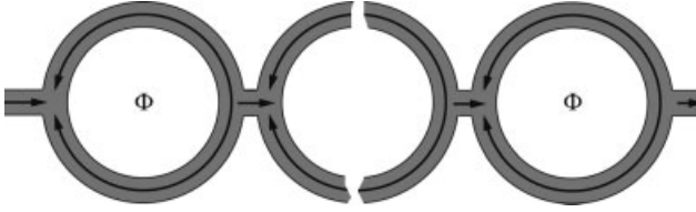
Figure 1.12 A series of interconnected ring-shaped conductors. Each ring is penetrated by a magnetic flux \Phi . The interference of the time-reversed trajectories leads to the Al'tshuler–Aronov–Spivak oscillations as a function of a magnetic field.
