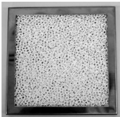
Figure 3.38 \text{TiO}_2 -coated porous ceramic filters for use as air filters. (Reprinted with permission from A. Fujishima, X. T. Zhang, Comptes Rendus Chimie 2006 , 9, 750).
