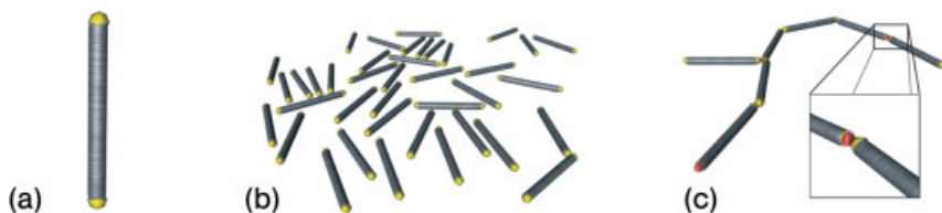
Figure 5.39 Schematics of dumbbell-like structures of a CdSe nanorod with Au gold tips at both ends. Single CdSe dumbbell doubly tipped with Au nanoparticles (a); typical unordered arrangement of Au tipped CdSe nanorods, where the Au tip size can be varied by increasing the \text{AuCl}_3 concentration during tip growth (b); self-assembled chain of nano CdSe dumbbells (real size 29 \times 4 nm) formed by adding hexanedithiol bifunctional linker molecules which connect Au tipped ends of CdSe dumbbells. Adapted from Ref. [110].
