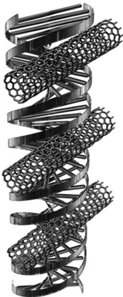
Figure 5.23 Theoretically proposed DNA–CNT composite structure. The single-wall CNTs are intercalated within the major groove of DNA. Adapted from Ref. [73].
