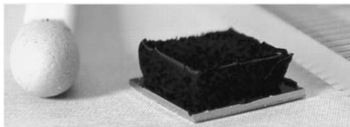
Figure 2.18 Shown are 2.5-mm-tall SWCNTs made by water-assisted ethylene CVD. A matchstick on the left-hand side of the picture shows the height of the nanotubes. The nanotubes have individual diameters of 1 to 3 nm and have grown to reach an aspect ratio of 10^6 , virtually unheard of for crystalline materials. (Reprinted with the permission of Hata, K. et al., Water-assisted highly efficient synthesis of impurity-free single-walled carbon nanotubes, Science 306, 1362–1364, 2004.)
