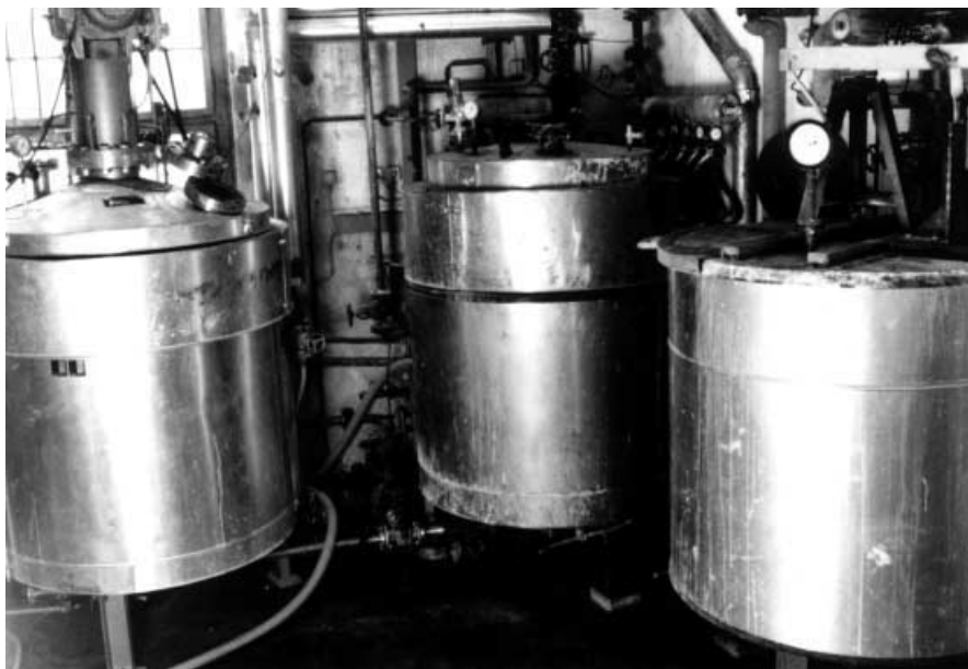
Fig. 4. Photograph of a semi-commercial plant for zeolite synthesis. Left is the stirred, pressurized reactor, middle is the pressurized reactor with heating coils, and right is the open reactor with heating coils and stirrer
