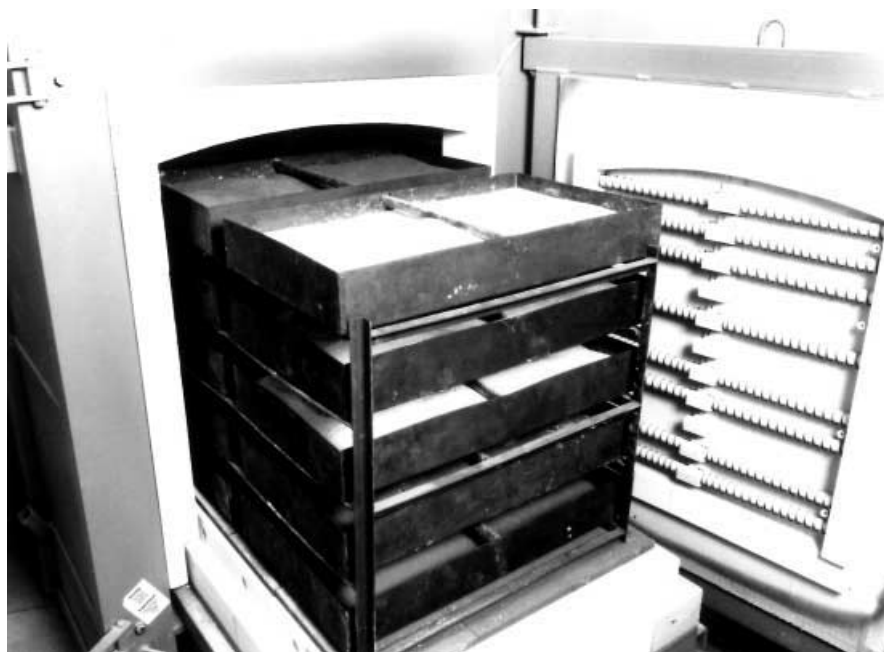
Fig. 5. Muffle oven of the semi-commercial plant to dry and calcine the zeolites after synthesis and filtration
