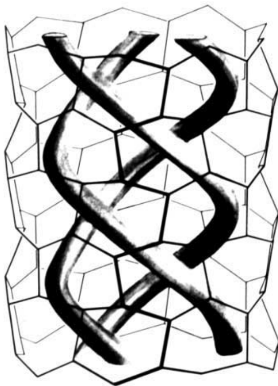
Fig. 10. The triple water helix, represented by the three grey tubes, within the 18-ring channel in VPI-5. Reproduced by permission of Elsevier Science from [19]
