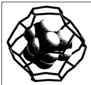
Fig. 26.3. TMA + cations occluded in the sodalite cage. In this representation, the T elements (T = Si, Al, etc.) making up the cage are located at the intersection of the edges and the oxygens atoms in the middle of the edges
