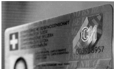
Fig. 29.22. Identity card protected from forgery by depositing alternating layers of inks with very different refractive indexes, using the OVI technique [14]
