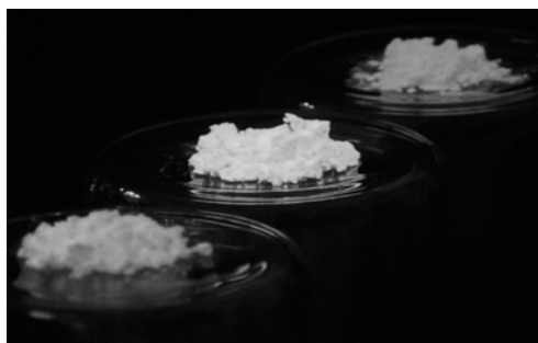
Fig. 29.3. Phosphors re-emit in the visible after UV excitation. See also the colour plate
