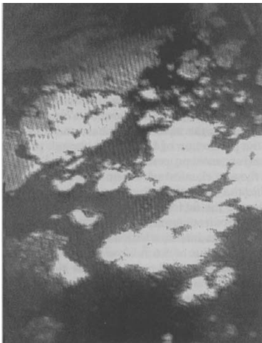
Figure 6.1. Brewster angle microscopic image of a pristine C_{60} layer on water; domains observed at \Pi = 0 \text{ mN m}^{-1} (the length of the image shown is 200 \mu\text{m} ).
