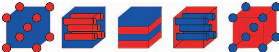
FIGURE 2.6. Block copolymer morphologies obtainable via phase separation. The exact structure will depend on the relative volume fractions of the two blocks, as well as \chi N (where \chi is the interaction parameter and N the length of the polymer).
