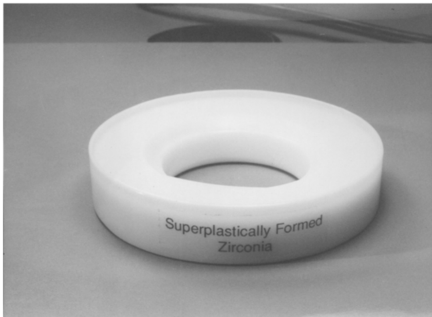
FIGURE 9.2 A plastically forged ceramic component molded from a nanostructure, dense preform. The forming operation was performed at 1400 C in less than 15 minutes. Used with permission from Nanomaterials: Synthesis, Properties and Applications , edited by A. S. Edelstein and R. C. Cammarata, 1996, IOP Publishing.
