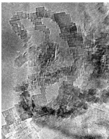
FIGURE 4.11 High-resolution TEM of AP-MgO. Note the cubelike nanocrystals that amalgamate into polyhedral structures with many corner/edges, and the embryonic pore structure. Reprinted with permission from J. Am. Chem. Soc. , 2000 , 122, 4921–4925. Copyright 2000 American Chemical Society. 113
