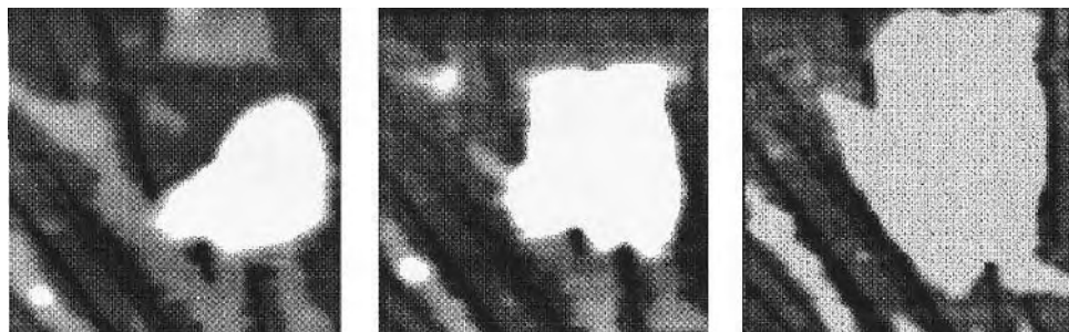
FIG. 20 Dewetting of Zdol-TX on a nonuniformly covered surface. As in the previous figure, bare substrate regions are exposed (darker areas). Only material in layer 2 dewets to form a droplet (bright area). Diffusion of molecules from layer 2 occurs on top of layer 1 and does not fill the uncovered, possibly contaminated, substrate regions. (From Ref. 70.)
