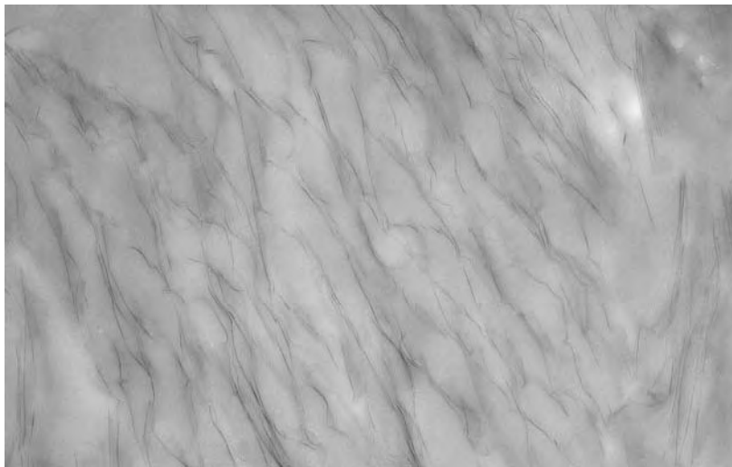
FIG. 7 TEM of polystyrene–montmorillonite nanocomposite. (From Ref. 45.)
