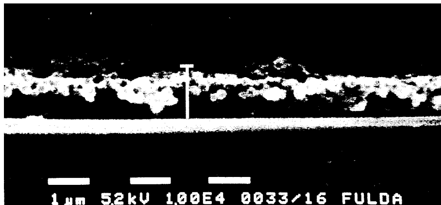
FIG. 21 Cross section of sample subjected to 10-fold alternating dipping into dispersions of 1b (5 \times ) and 2 (5 \times ). The bar indicates the average particle film thickness of 1.2 \mu\text{m} . (From Ref. 93, with permission from Elsevier, Amsterdam.)
