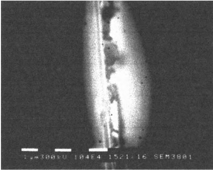
FIG. 43 SEM image of PbS–CdS–PbS superlattice.
