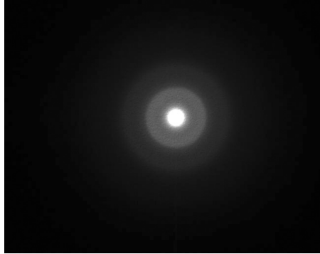
Fig. 4.18. SAD pattern (where there is no crystallite) of nc-TiN/a-SiN x nanocomposite thin film with 11.3 at.%Si (sample P4) showing a diffuse pattern typical of an amorphous phase.
