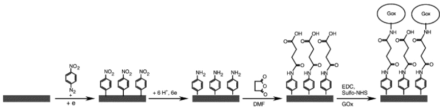
Fig. 3.14. Schematic drawing of covalent immobilization of glucose oxidase on diamond surface [91].
