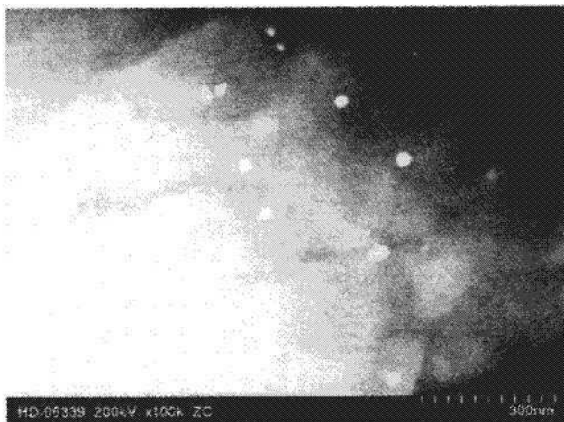
Figure 1. Dark-field TEM image of aggregated large gold particles on mesoporous \text{SiO}_2 (SBA-15) [22]. The sample was prepared by deposition-precipitation of \text{Au}(\text{OH})_x\text{Cl}_{4-x}^- directly on SBA-15. Reproduced with permission of the American Chemical Society from Supporting Information of W. F. Yan, B. Chen, S. M. Mahurin, E. W. Hagaman, S. Dai and S. H. Overbury, J. Phys. Chem. B 108, 2793 (2004).
