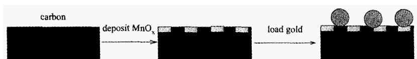
Figure 10. Schematic representation for the synthesis of Au/MnO x /C catalysts, including Au/MnO x /mesoporous carbon, active for CO oxidation [34]. The carbon surfaces were decorated by MnO x via an electroless-deposition method, and gold nanoparticles were subsequently loaded onto MnO x /C. Reproduced with permission of Elsevier from Z. Ma, C. D. Liang, S. H. Overbury and S. Dai, J. Catal. 252 , 119 (2007).
