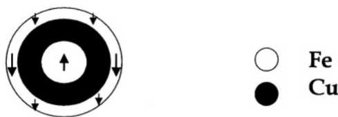
Figure 17. Antiferromagnetic coupling observed in Fe@Cu@Fe multilayer nanoparticles. Size of the successive layers: 8 nm, 10 nm and 11.4 nm, respectively.
