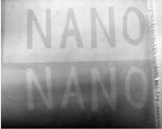
Figure 5.11 Polyester fabric modified with a photochromic nanosol coating. The sample was masked with a pattern (positive and negative) and irradiated with a UV-lamp. Photograph was taken immediately after irradiation, since the color will completely fade within minutes.
