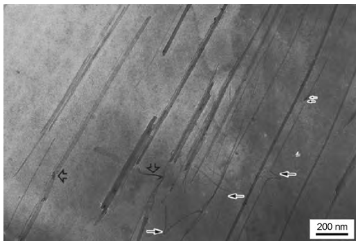
Figure 1.36 Alignment of nanotubes in a polymer matrix following cutting with microtome: arrows indicate buckled nanotubes (Reproduced from ref. 68)
