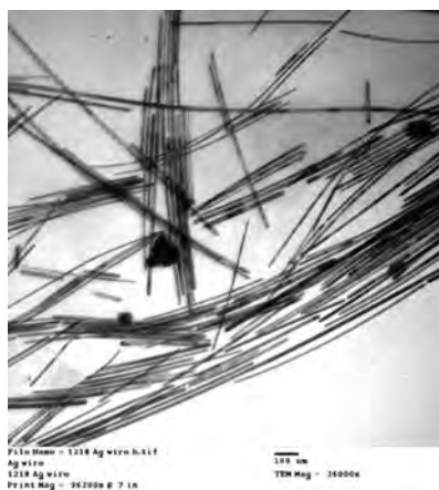
Figure 3.22 TEM images of Ag nanowires obtained using the procedure outlined in ref. 153 (Reproduced from ref. 153)
