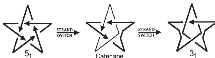
Figure 2.7 A knot–catenane–knot conversion; a 5_1 knot is converted to a catenane after two strands in a crossing exchange of their outgoing partners, the catenane converts to a trefoil knot with another exchange, (reproduced with permission from Seeman, N. C. DNA Nanotechnology: Novel DNA Constructions. Annu. Rev. Biophys. Biomol. Struct. , 27 , 225–248 (1998)).
