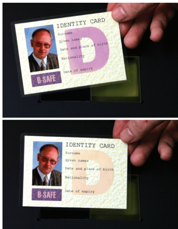
Figure 2. ID card sample in which the symbol “D” is printed with a BR-based ink. Top—initial color after storage; bottom—color after flashing with light.
