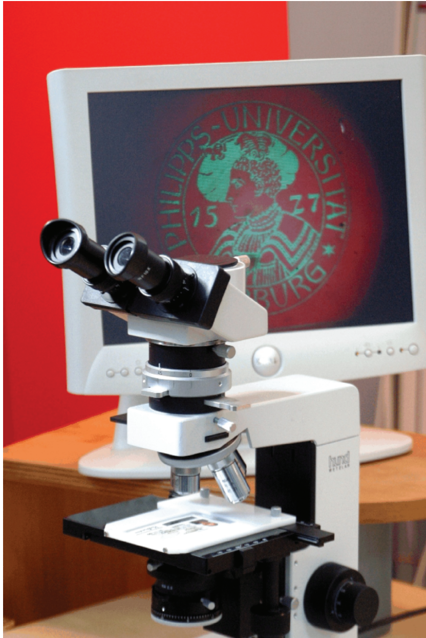
Figure 3. Optical data storage in an ID card sample made from BR-inks. In the microscope and on the screen, the stored seal of the University of Marburg is seen.
