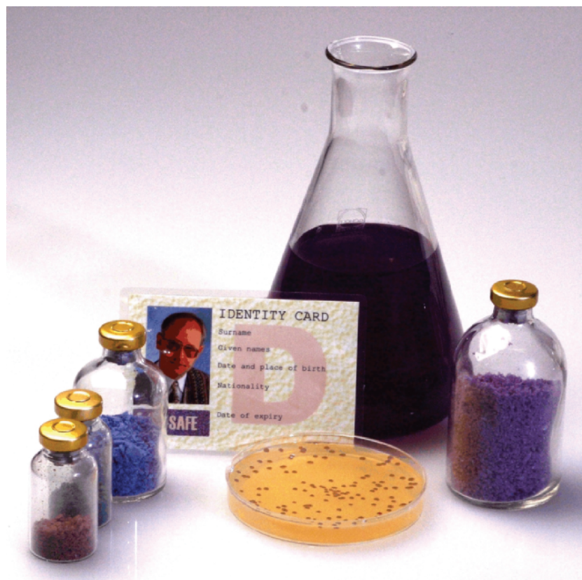
Figure 4. From the clone to the product. Clones of H. salinarium on the petri dish and isolated BR in the Erlenmeyer flask. Lyophilized BR and variants with different colors are shown in the sample vials. An ID card, as shown in Fig. 2, made using BR-based inks is positioned in the middle.
