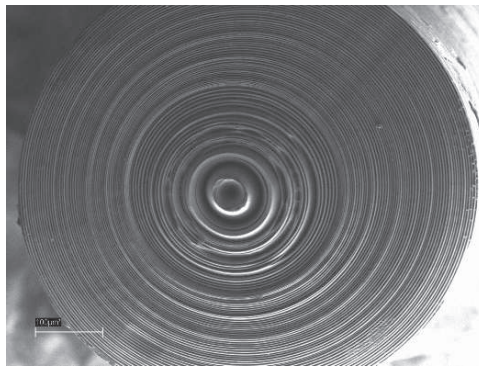
Fig. 4 Photo of Hyalonema siebody basal spicule end-face, etched in HF solution and polished, obtained by scanning electron microscopy (scale 100 \mu\text{m} )
