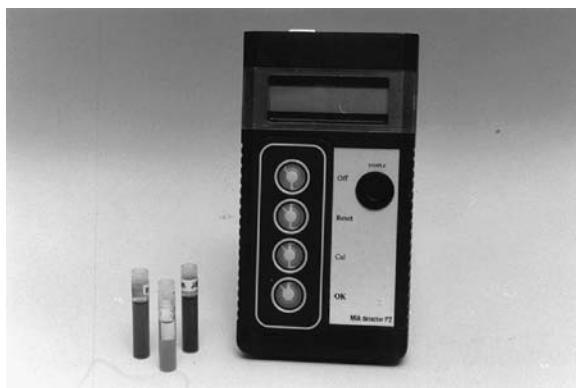
FIGURE 7.6 The current magnetic permeability meter, a portable version of the device (21)
