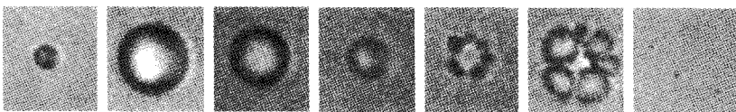
Fig. 9. In the images above, a single 3 \mu\text{m} bubble is shown (far left) in the resting state. Insonation with a single pulse of ultrasound energy causes the bubble to expand, collapse, and fragment, yielding nanometer-sized fragments. As the bubbles expand and collapse, they generate a local shockwave that can be used therapeutically. Reproduced with permission from Chomas et al., Appl Phys Lett , 2000. 30
