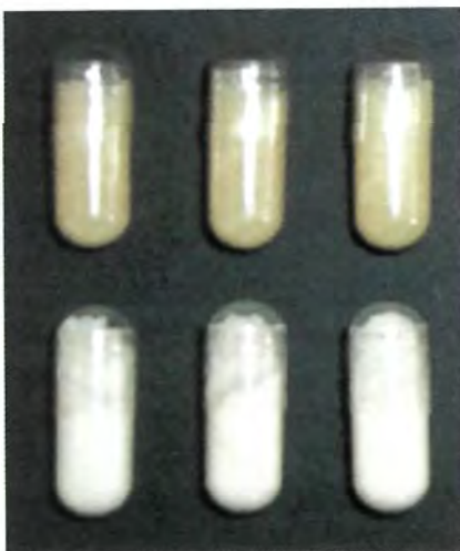
Fig. 5. Gelatin capsules filled directly with hot liquid PEG nanosuspension, solidification takes place in the capsules (upper) or filling of the capsules with milled solidified PEG nanosuspension (lower). (From Ref. 36 with permissions.)
