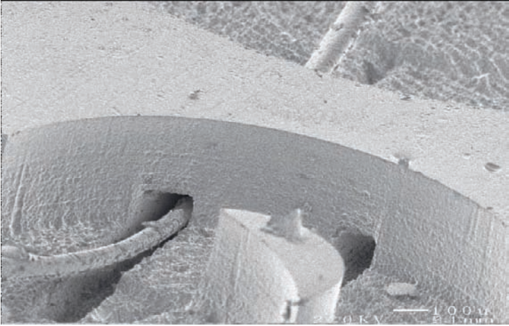
Figure 2. Scanning electron microscope photograph of an embedded channel etched between two fluidic chambers. A human hair has been threaded between the chambers.
