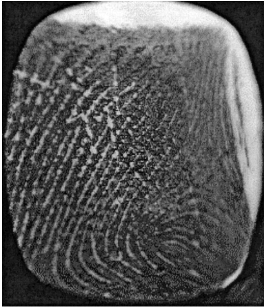
Figure 11.10 SED image of the fingerprint on gold from the Auger system has a three-dimensional effect. At low magnification the whole fingerprint was visible. The image remained unchanged with the electron beam on the same area for over one hour without any noticeable effects.
