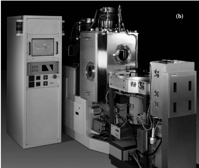
Figure 4.29 Photographs of GCIB systems: (a) is an early system fabricated for university research; (b) is a unit of the commercial type sold to microelectronic manufacturers.
