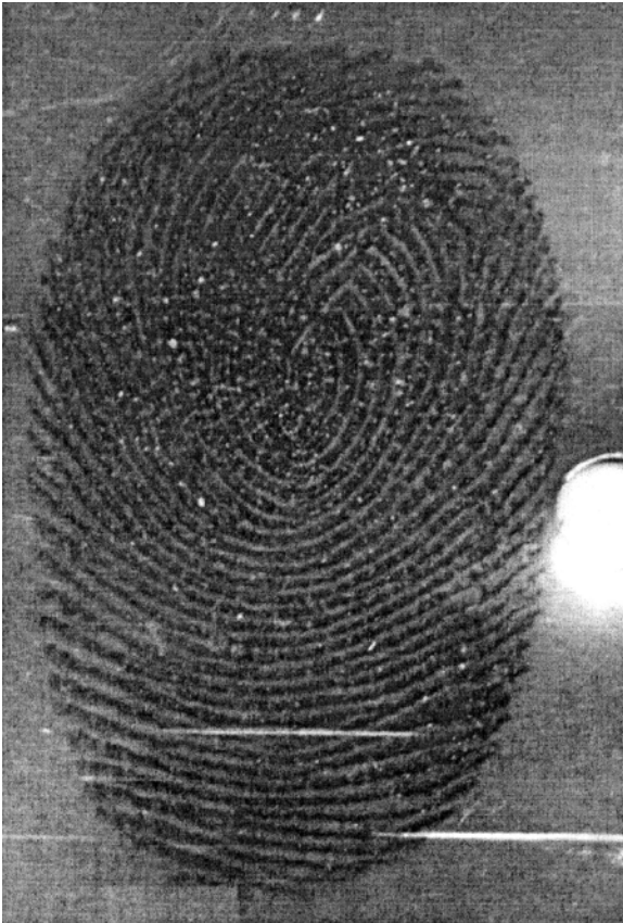
Figure 11.3 A fingerprint was placed on a metal strip of 5000 Å of gold over stainless steel. After implantation the fingerprint appeared very dark and could be rubbed without smearing.
