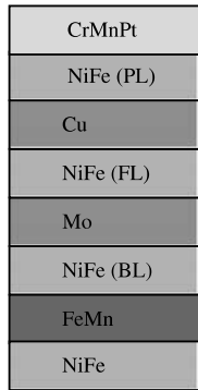
Fig. 3. Schematic of spin valve sensor with interlayer exchange coupling domain bias scheme
