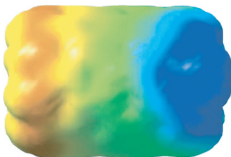
Figure 2 Computed (HF/STO-5G//STO-3G) electrostatic potential V_S(\mathbf{r}) on the outer surface of the (8, 0) C_{80}H_{15}NH_2 model carbon nanotube. The NH_2 group is at the right end. The variation in V_S(\mathbf{r}) is between -26.1 kcal/mole at the left end and +26.1 kcal/mole at the right
