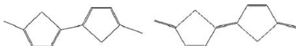
FIGURE 21.18 Unit cells of the two isomers of the infinite thiophene. On the left is the benzenoid; on the right, the quinoid configuration. (From G. Speyer, R. Akis, and D.K. Ferry, J. Vac. Sci. Tech. B , 24(4), 1987–1991, 2006. With permission.)
