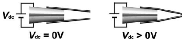
Fig. 9.15 Schematic of nanotube nanotweezers. Two carbon nanotubes are attached to two independent electrodes deposited on a glass micropipette. The nanotweezers are closed by applying a voltage between the electrodes. (From [97]. Reproduced with permission from AAAS)
