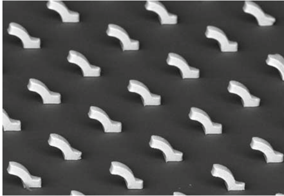
Fig. 22.21 Spring-like compliant interconnects used to minimize stress coupling between the silicon and package
