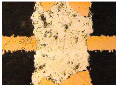
Fig. 11.2 Photograph of a cross section showing a conductive adhesive in a microvia. In this instance, interconnection is made vertically between copper pads, and laterally to a copper inner plane
