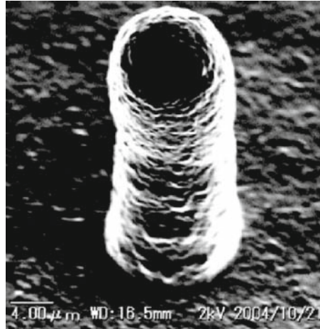
Fig. 12.17 SEM image of a gold pillar with diameter of about 6 \mu\text{m} fabricated by superfine inject system on silicon substrate [43] (with permission)
