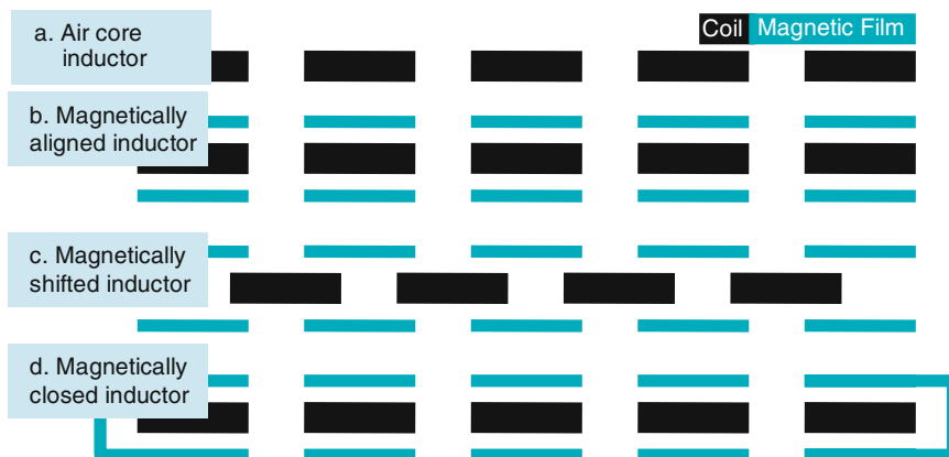
Fig. 9.8 Cross-sectional view of relative position of magnetic film with respect to the spiral leg [10]
