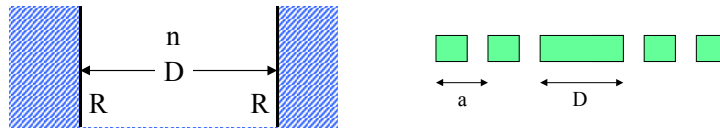
Figure 1.19. Microcavity or defect in a 1DPC, formed in a dielectric waveguide
