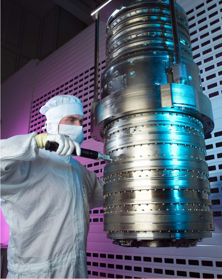
Figure 1.3 A photolithography projection lens assembly (Courtesy: ASML Corporation).
