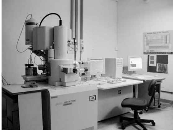
Figure 1.12 A Field Emission Scanning Electron Microscope, a common high-resolution tool for surface analysis. Photo courtesy of the Plasma Sources and Applications Center of Nanyang Technological University, Singapore.
