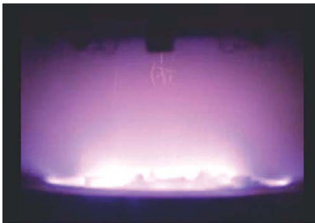
Fig. 6.2 A typical plasma glow in the process of the plasma-assisted co-sputtering deposition of bioactive hydroxyapatite coatings.
