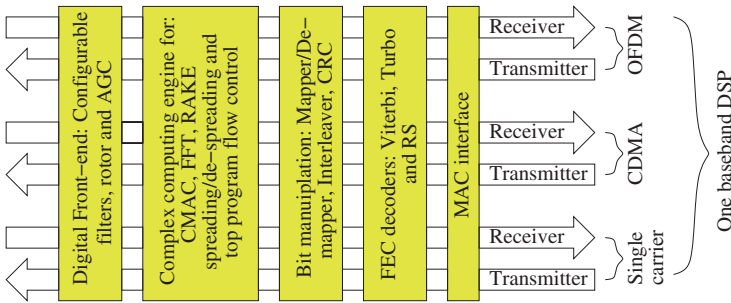
Figure 5.4. Hardware multiplexing on LeoCore DSPs.
