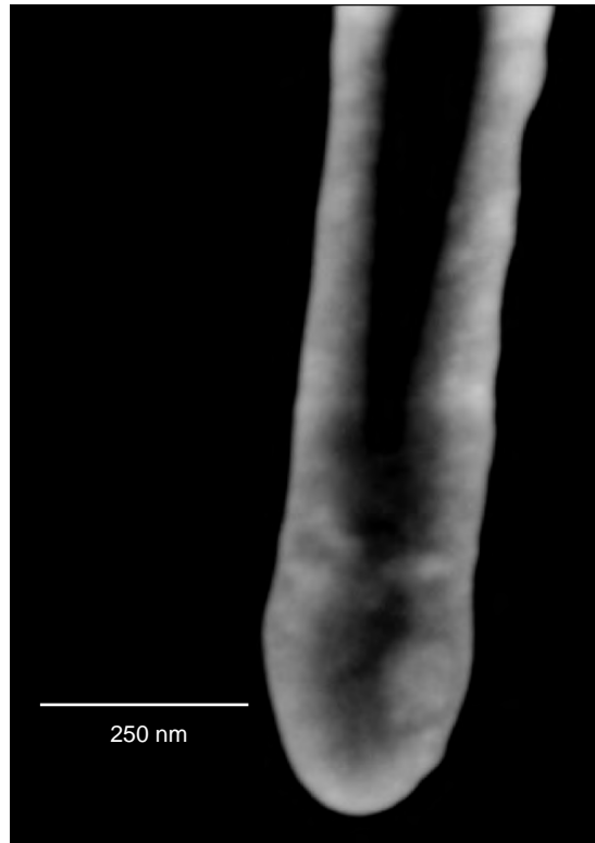
FIGURE 7.8. TEM micrograph of an oxide-coated tungsten probe. The tungsten is the darker material encased in the lighter colored oxide. The sharpness of the probe will increase on the order of 80% with the complete removal of oxide. (Adapted from [22].)
