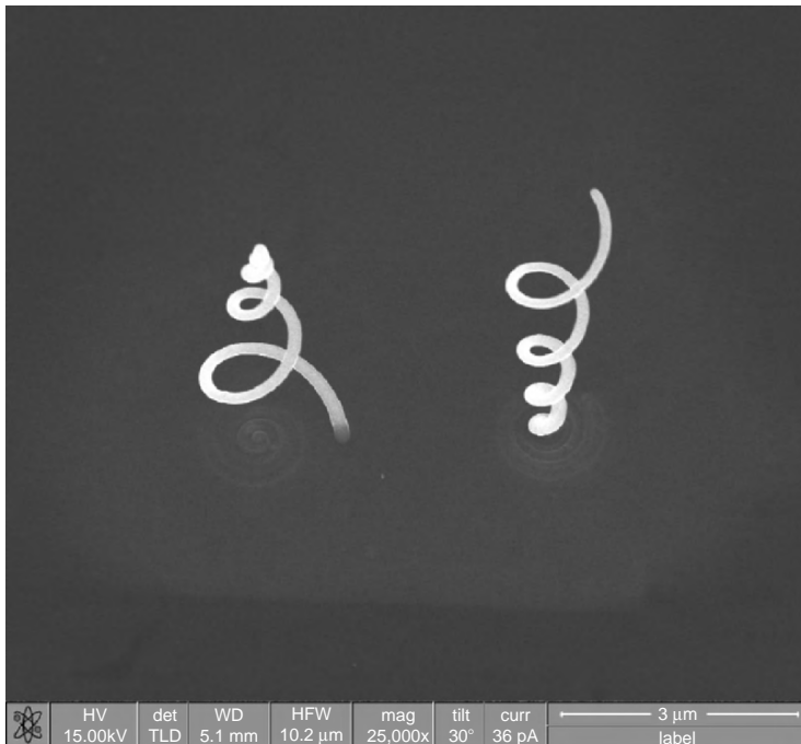
FIGURE 8.12. SEM image of 3D free-standing Pt FIB deposited growth. (Image courtesy of S. Reyntjens.)
