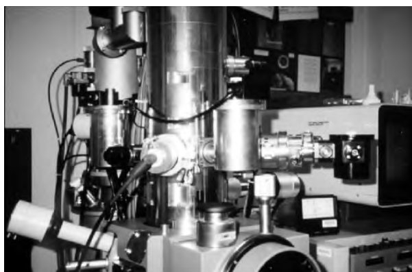
FIGURE 15.7. A JEOL 7401 near-lens FESEM is designed to accommodate the attachment of a cryochamber.
