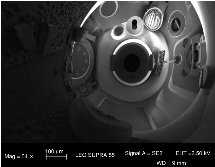
FIGURE 4.5. A secondary electron image formed by charging a plastic sphere at 20 kV, and then imaging the sample at 2.0 kV. The resulting image is formed by the low kV primary beam being reflected about the chamber by the sample that has been charged to a higher kV.
