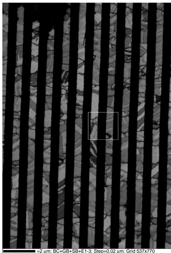
FIGURE 2.32. All-Euler orientation map with grain boundaries. Most grains are heavily twinned and span the length of interconnect lines. Drawn box shows location of higher-resolution run. Scale bar = 2 \mu\text{m} (see color insert).
