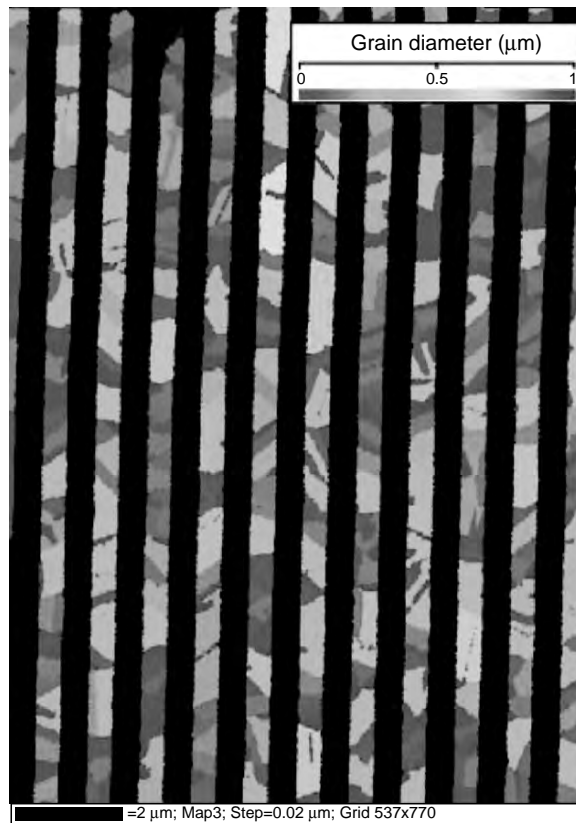
FIGURE 2.34. Grain size (equivalent-circle diameter) map, with all \Sigma 3 twins as grain-delimiting boundaries. Scale bar = 2 \mu\text{m} (see color insert).
