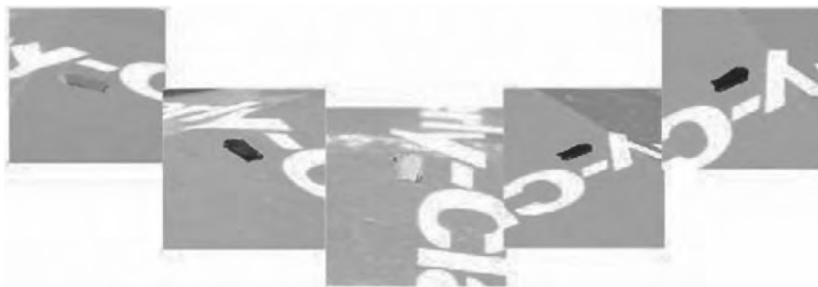
FIGURE 12.22. Color changes of photonic-crystal metal-mesh composites as a function of angle. The thin composite piece is displayed on green paper with a line of text to help indicate changes in orientation. The observed colors are green, brown, yellow, and blue and black, for the relative orientation angle of 30^\circ , 60^\circ , 90^\circ , 120^\circ , and 150^\circ , respectively. Red, purple, and other colors (not shown) can also be observed at other angles (see color insert).
