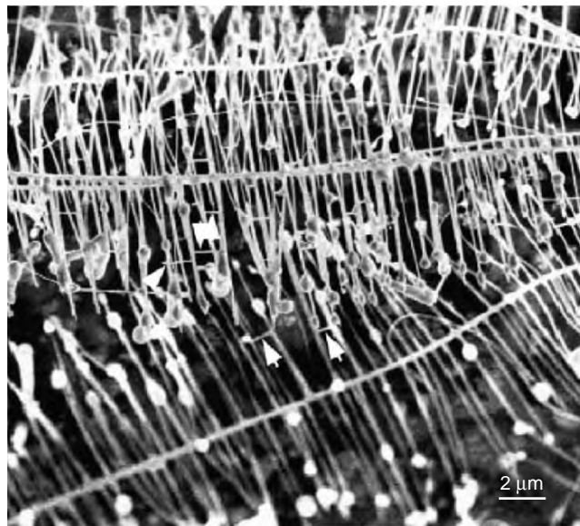
FIGURE 1.18. SEM image of \text{SnO}_2 nanojunctions showing depth of field.
