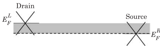
Figure 2.15 Transport of electrons in the shaded band between the drain and source Fermi energies leads to an excess kinetic energy, which gives rise to kinetic inductance in addition to magnetic inductance.
