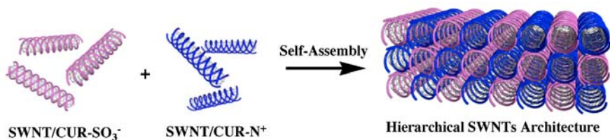
Fig. 38 Proposed concept for creating hierarchical SWNT architecture from one-dimensional building blocks through electrostatic interaction. It should be noted that all processes including wrapping of SWNTs by CUR and self-assembling of the resultant composites proceed in a supramolecular manner. Reprinted with permission from [199]
