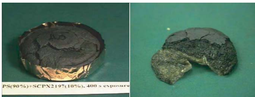
FIGURE 3.8 Image of a PS/mass fraction 10% MMT nanocomposite pyrolyzed for 400 s. The image on the right shows a cross section and partial removal of the surface char.
