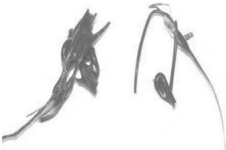
FIGURE 12.5 Polyamide-6 nanocomposite after 1 min of processing (purple, intercalated) and 7 min of processing (red, exfoliated). (From Ref. [98].) (See insert for color represent of figure.)
