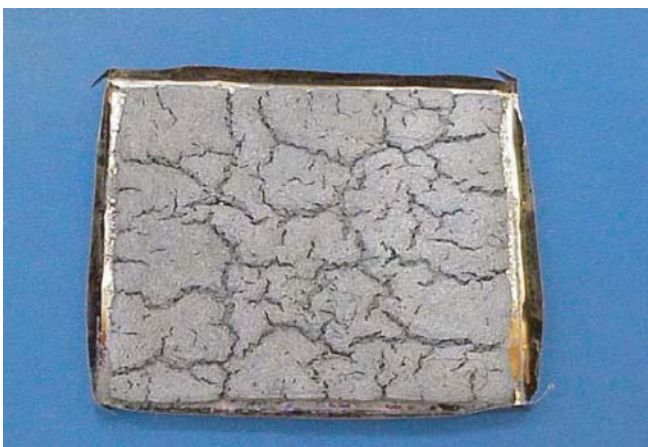
FIGURE 3.17 Gasification residue of PP/PP-g-MA/synthetic hectorite with 7.7% PP-g-MA and hectorite.
