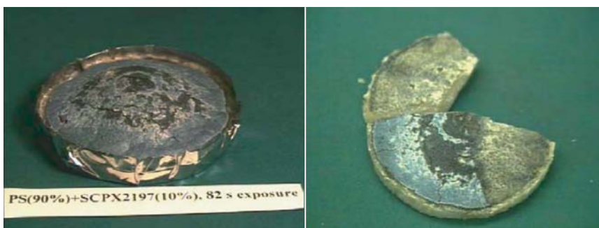
FIGURE 3.5 Image of a PS/mass fraction 10% MMT nanocomposite pyrolyzed for 82 s. The image on the right shows a cross section and has had the surface char partially removed.
