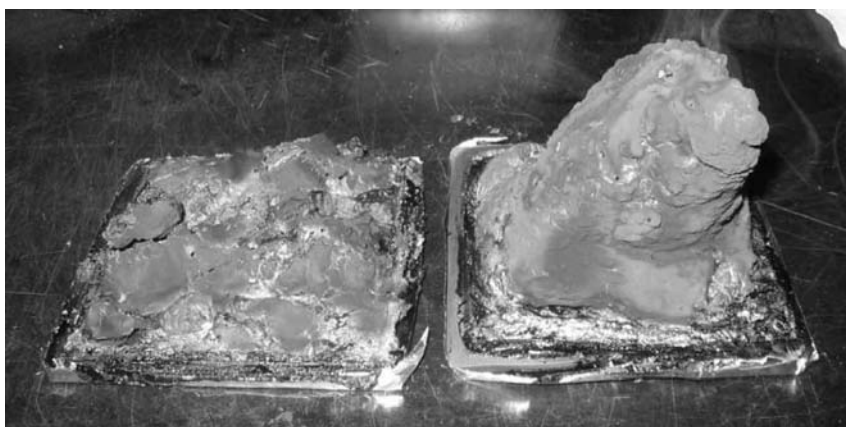
FIGURE 9.29 Residue after a cone calorimeter test of laminate PP–GF coated 1 mm thick: on the left side a standard epoxy–APP formulation (microcoat), and on the right side an LDH modified formulation (nanocoat). (Courtesy of Consorzio CETMA, Italy.)
