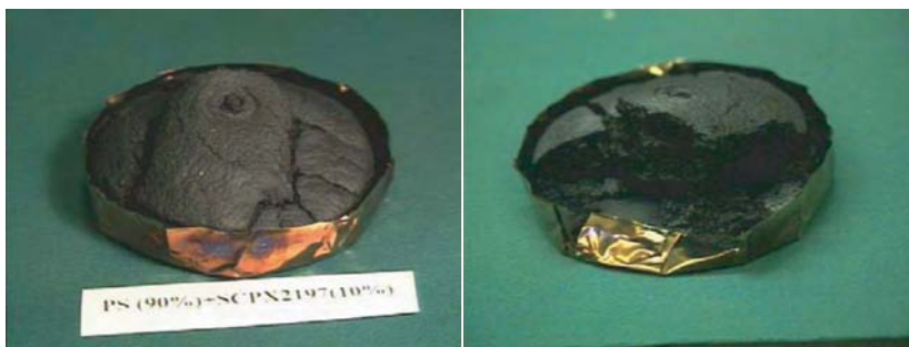
FIGURE 3.9 Image of a PS/mass fraction 10% MMT nanocomposite pyrolyzed for 1150 s. The image on the right shows a cross section and partial removal of the surface char.
