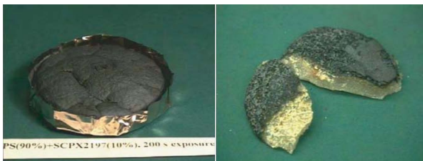
FIGURE 3.7 Image of a PS/mass fraction 10% MMT nanocomposite pyrolyzed for 200 s. The image on the right shows a cross section and partial removal of the surface char.
