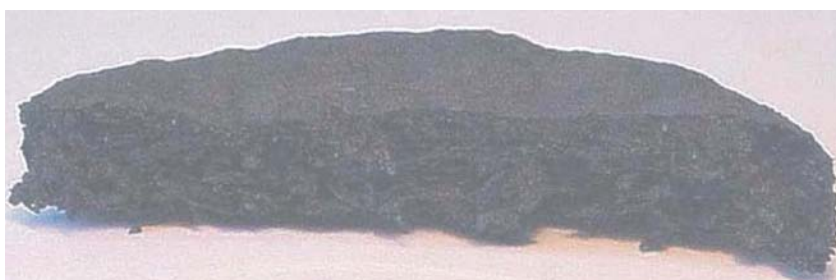
FIGURE 10.27 Cross section of the residue of PP-MWNT (1%).
