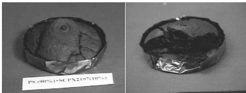
FIGURE 3.9 Image of a PS/mass fraction 10% MMT nanocomposite pyrolyzed for 1150 s. The image on the right shows a cross section and partial removal of the surface char. (See insert for color representation of figure.)
