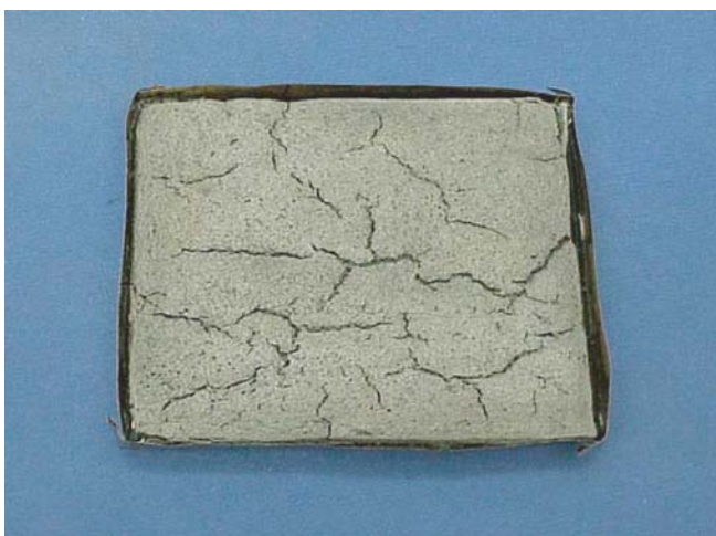
FIGURE 3.16 Gasification residue of PP/PP-g-MA/MMT with 7.7% PP-g-MA and MMT.
