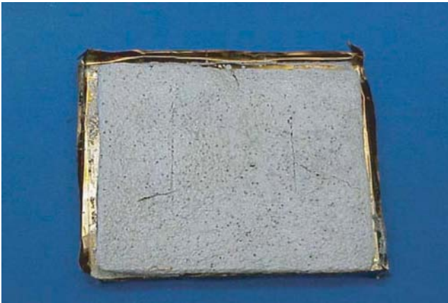
FIGURE 3.18 Gasification residue of PP/PP-g-MA/synthetic mica with 7.7% PP-g-MA and mica.
