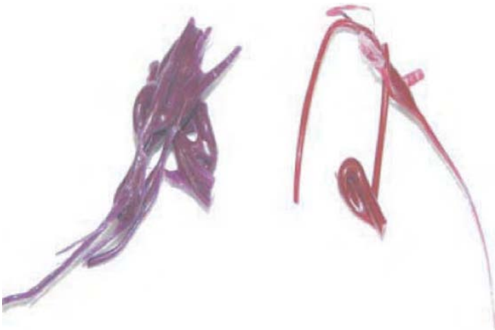
FIGURE 12.5 Polyamide-6 nanocomposite after 1 min of processing (purple, intercalated) and 7 min of processing (red, exfoliated). (From Ref. [98].)
