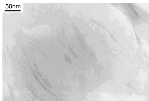
FIGURE 8.2 HREM of ABS-OMT nanocomposite. (From Ref. 35, copyright © 2004, Elsevier, with permission.)
