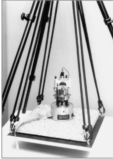
Fig. 1.2. Ready-to-use vibration protected typical AFM (Nanoscope III) with stage, including the XYZ -piezo unit, sample mount, cantilever tip, laser focused to the backside of the reflecting cantilever and guided to a split photodiode for the feedback loop that controls the constant force and provides the topologic information
